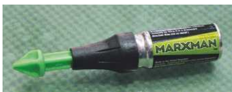
The Marxman is used for marking walls before drilling
